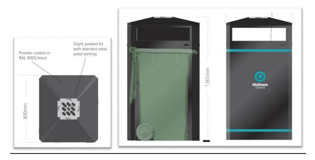
New proposed large capacity metal bin housings containing a standard 240 litre standard wheeled refuse bin.
